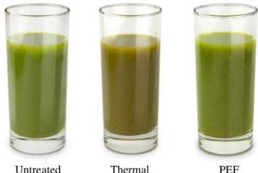
Figure 2.4 Color difference of untreated, thermally treated, and PEF-treated green smoothie (Elea, 2018). PEF: Pulsed electric field.
